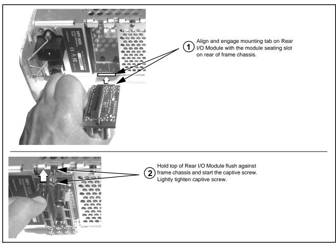
Figure 2-2 Rear I/O Module Installation
