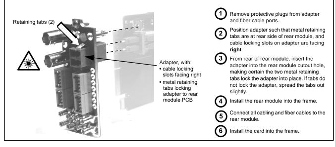
Figure 2-3 Fiber and Balanced Audio Connections
