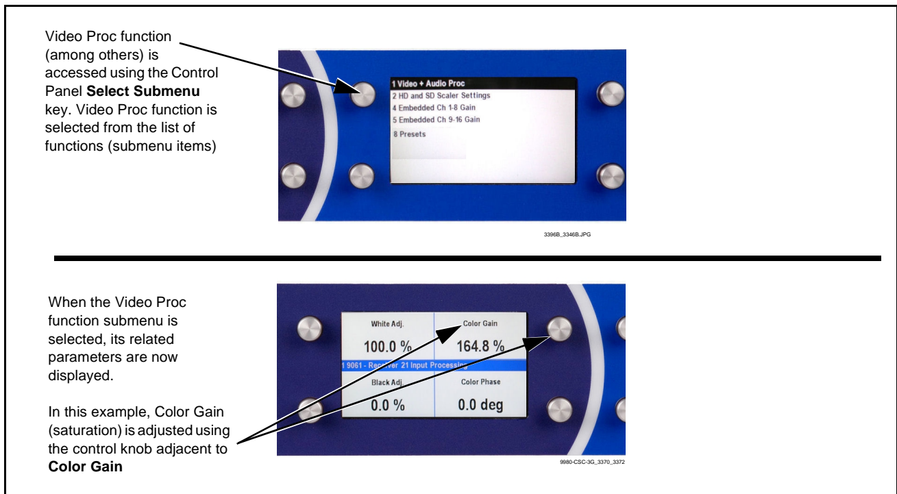
Figure 3-3 Remote Control Panel Setup of Example Video Proc Function Setup
