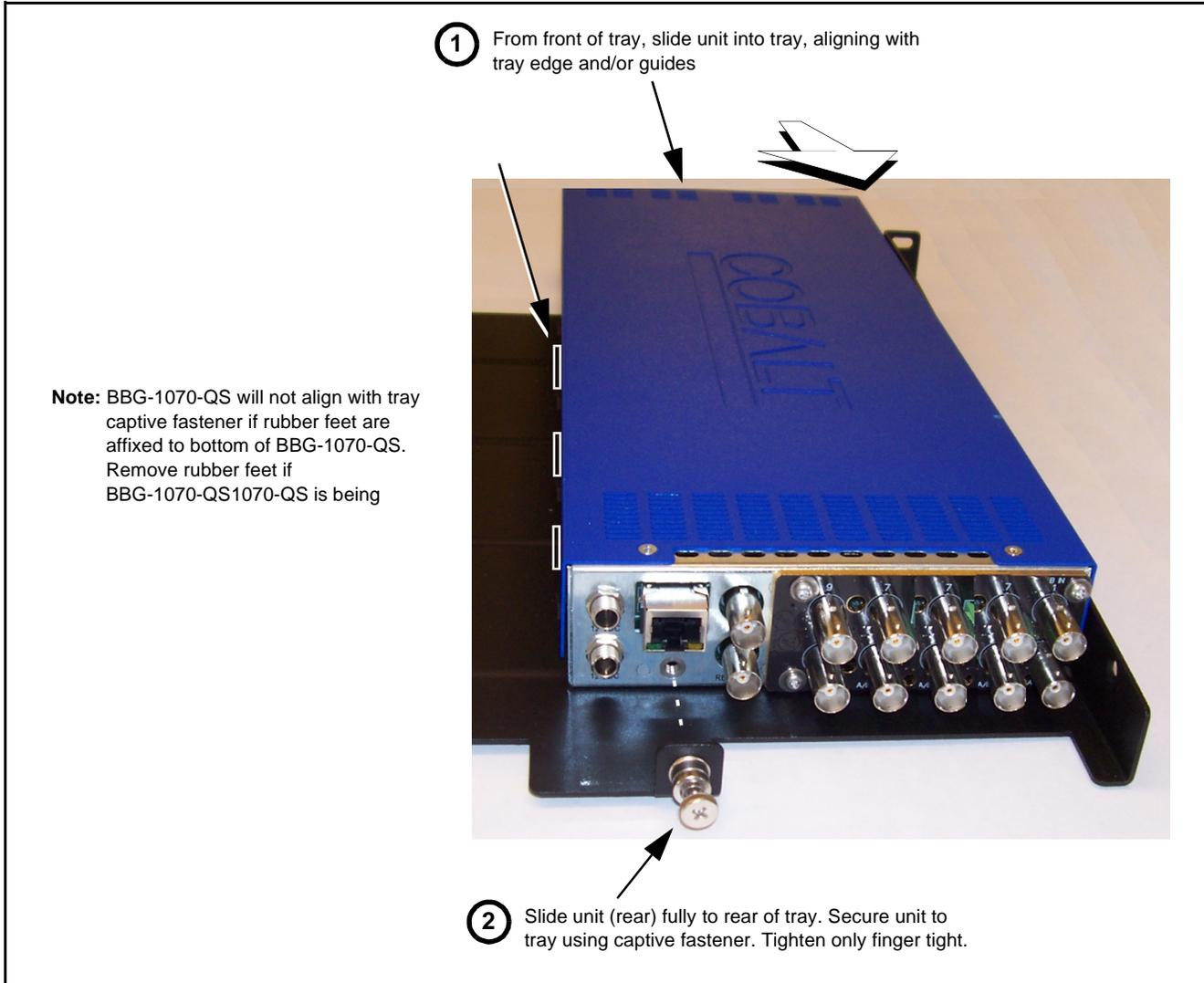
*Figure 2-1 Mounting BBG-1070-QS Using Frame Mounting Tray*
