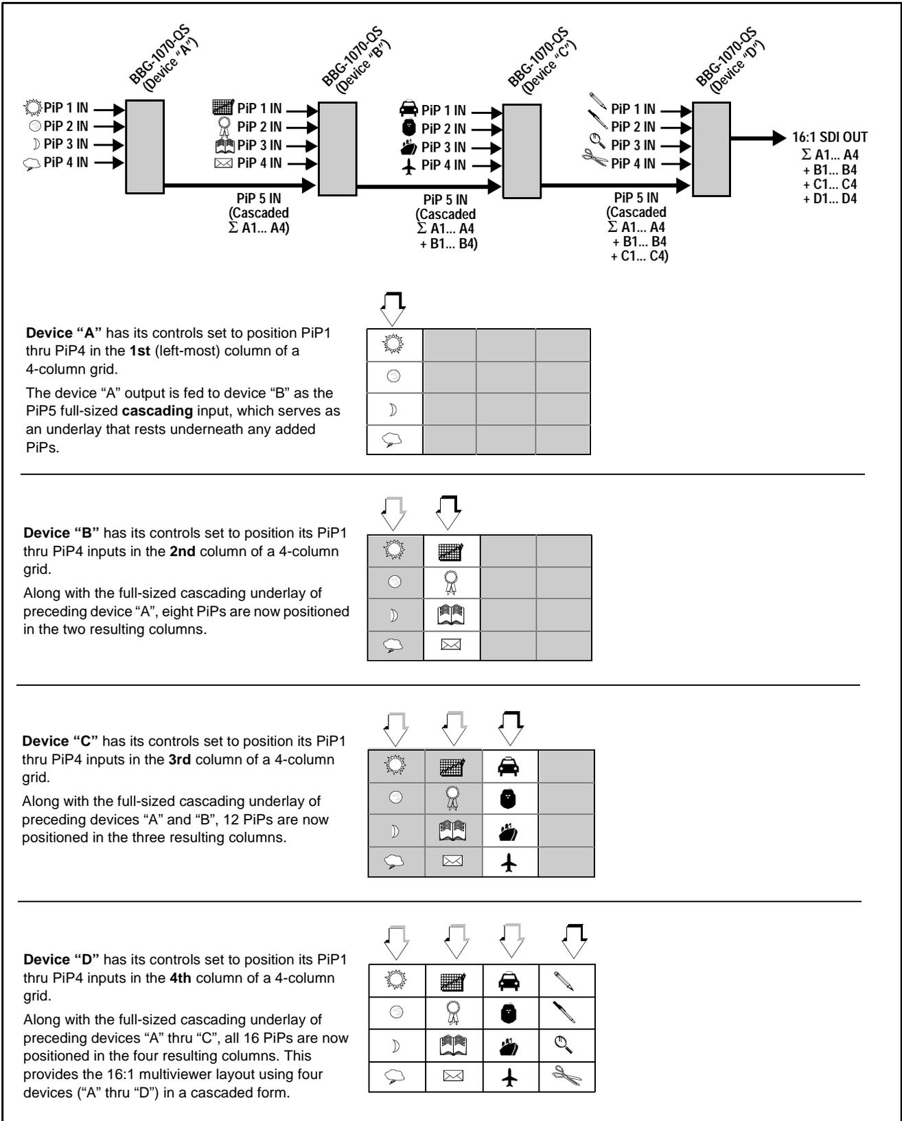
Figure 1-3 Cascaded BBG-1070-QS Example 16:1 Setup and Overview
