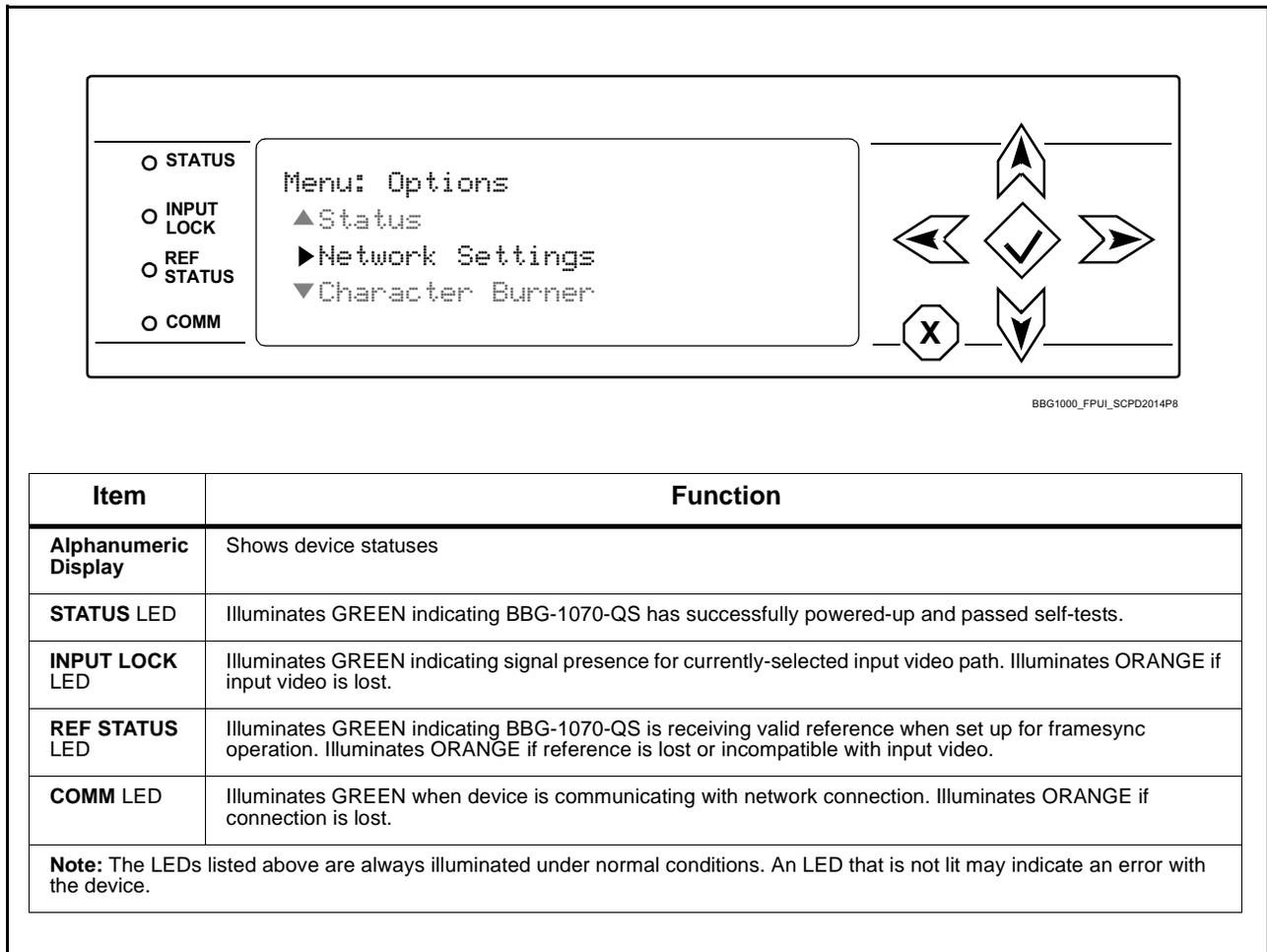
**Figure 3-8 BBG-1070-QS Device Edge Status Indicators and Display**
