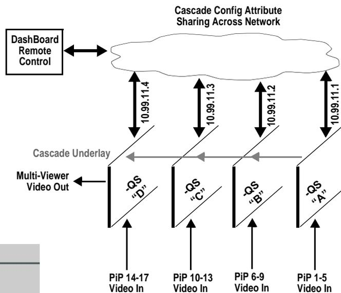
For each per-PiP control, the result is **all** PiPs within the chain being exposed, allowing settings to be performed from **any** of the units and cloned to any unit as desired. User presets can encompass all units in the chain and be invoked in a single action done at one unit.
