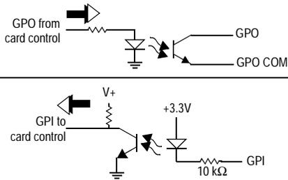
GPI uses equivalent opto-isolated circuits shown below.
