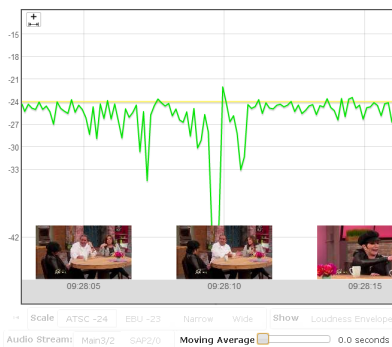
Zero-second moving average shows instantaneous LKFS excursions
