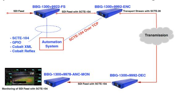
Cobalt offers a complete programmer-side Ad Insertion solution, ready to connect to your traffic system. Our ancillary data inserters and frame syncs can be licensed to add SCTE-104 triggers to an SDI signal, in a frame-accurate manner. These devices can be interfaced with your traffic system using the following options:
