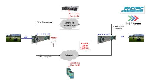
With the Reliable Internet Stream Transport (RIST), you can use your current Internet service for low-latency, reliable, secure content contribution – without being tied up to a vendor-proprietary solution. RIST is an open specification from the Video Services Forum and is currently widely available in the industry. RIST support in the Cobalt encoders and decoders combines all the best features of RIST in a single package:
