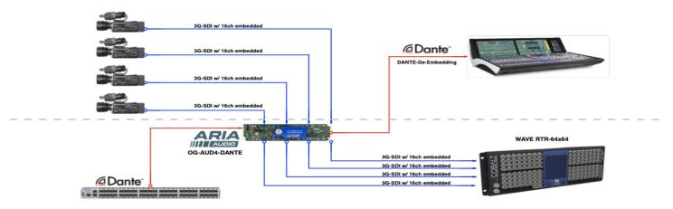
The new Cobalt ARIA OG-AUD4-DANTE card has four video paths supporting up to 12G SDI, as well as DANTE, AES, and MADI inputs and outputs. The card can simultaneously embed and de-embed audio between SDI, DANTE, AES, and MADI with flexible routing and mixing. It also includes a built-in frame sync.
