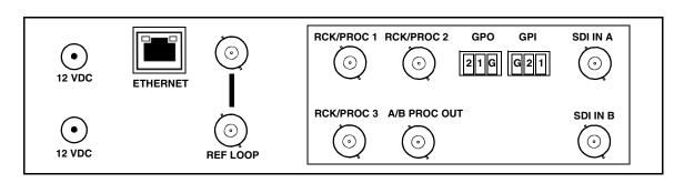
Note: A/B PROC OUT is the card processed output which uses either input SDI IN A or SDI IN B. This output uses relay latching to retain selected routing in the event of power loss regardless of whether a selection was manually invoked or by a unit-detected failover (for example, if an auto-changeover from A to B was invoked while active, routing of input B to this output is retained in the event of power loss).
