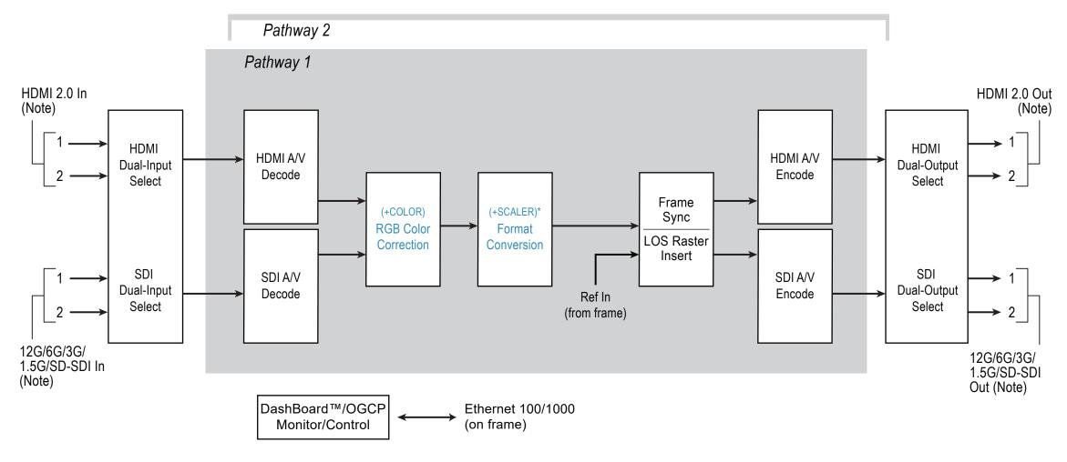
**Note:** Inputs can be selected from up to 2 discrete HDMI and 2 discrete SDI inputs. Dual simultaneous path processing is available with pathway 2 offering same features/functions as shown for pathway 1.
