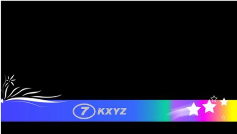
**Alpha Threshold** keying allows cost-effective luminance keying from low-cost generic file-based graphic sources. With the graphic source applied to both the card **Key** and **Fill** inputs, the card **Key Alpha** and **Key Threshold** controls can be set to easily optimize the key/fill as shown below.
