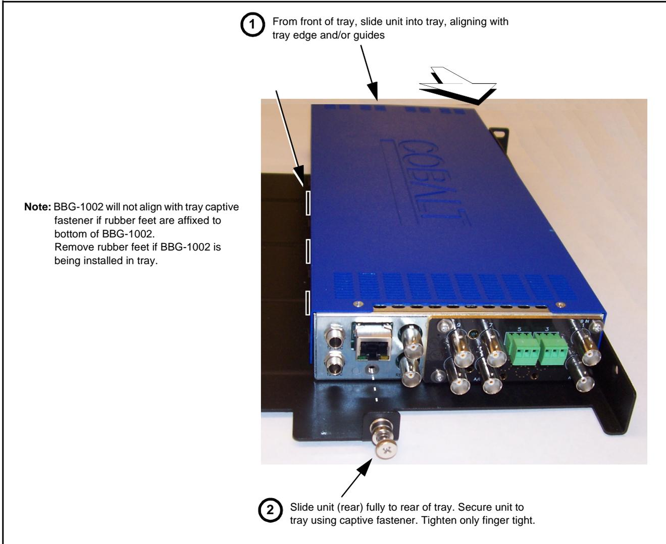
*Figure 2-1 Mounting BBG-1002-UDX-FS Using Frame Mounting Tray*
