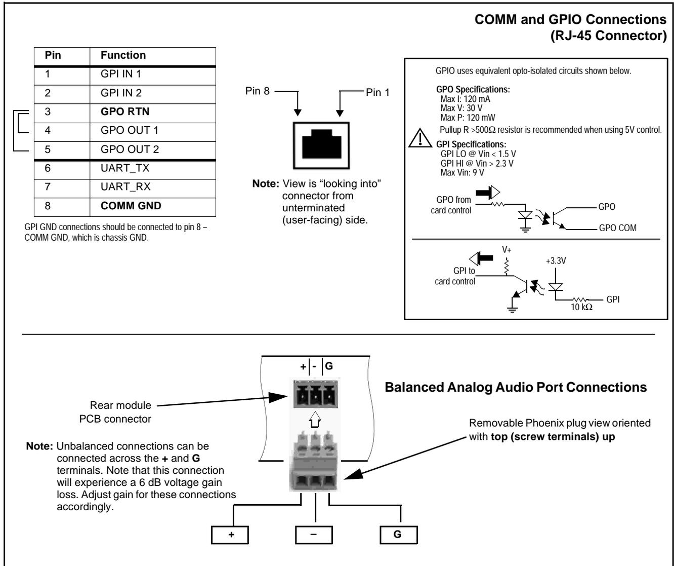
Figure 2-4 COMM, GPIO, and Analog Audio Connector Pinouts
