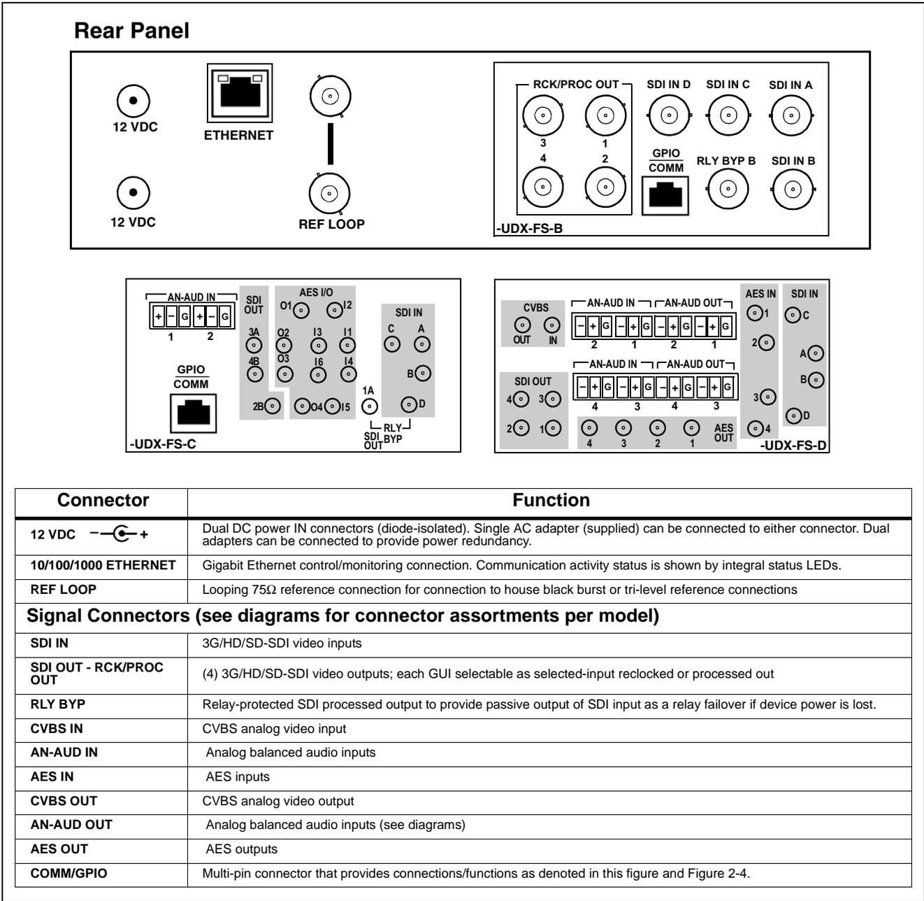
Figure 2-3 BBG-1002-UDX-FS Rear Panel Connectors
