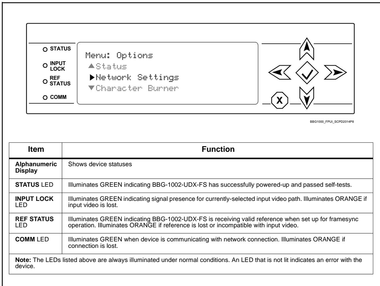
**Figure 3-9 BBG-1002-UDX-FS Device Edge Status Indicators and Display**
