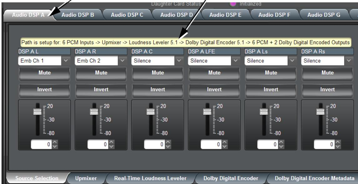
With the **Source Selection** sub-tab opened, we now assign the device basic input channels that the processing chain will use (in this example, sourcing from basic inputs Emb Ch 1/2). Since all of the processes selected here reside in DSP A, each process will forward its processed signal to the next enabled process in the DSP pipeline.
