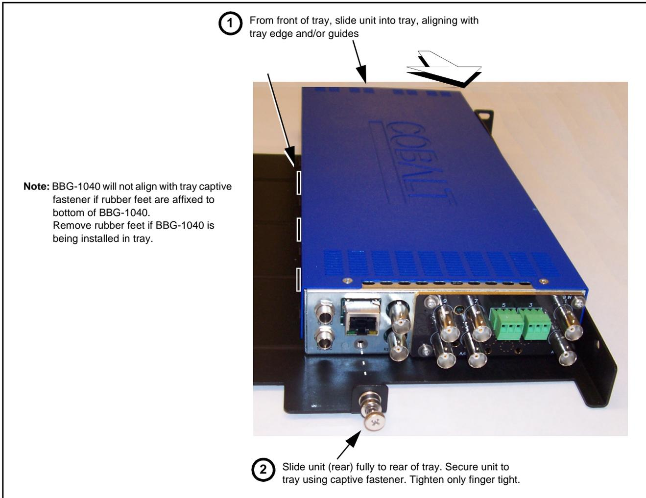
*Figure 2-1 Mounting BBG-1040-ACO Using Frame Mounting Tray*
