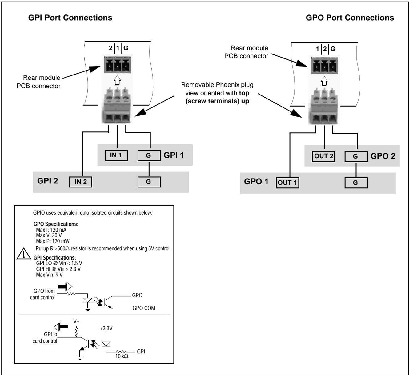
Figure 2-4 GPIO Connector Pinouts
