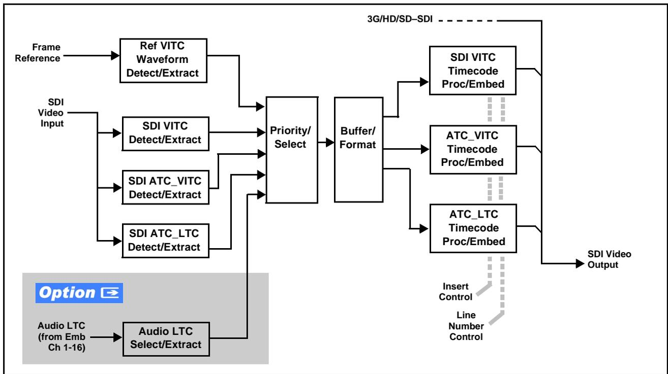
Figure 1-3 Timecode Processor
