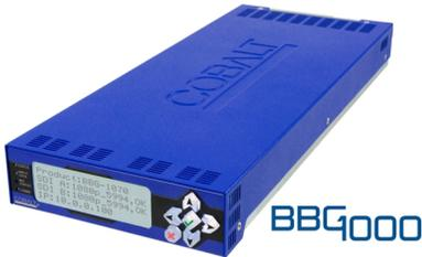
The Cobalt® **BBG-1070-QS 3G/HD/SD-SDI/CVBS Standalone Expandable Multiviewer with Advanced On-Screen Graphics** integrates five discrete 3G/HD/SD-SDI or CVBS inputs onto a single 3G/HD/SD-SDI quint-split output, with each input image being flexibly inserted into the output image area.
