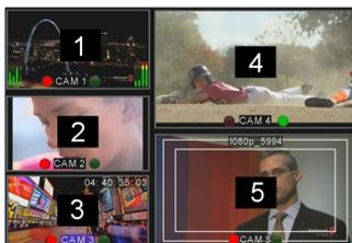
Pressing the Identify PiP button instantly correlates each image to its PiP channel.
