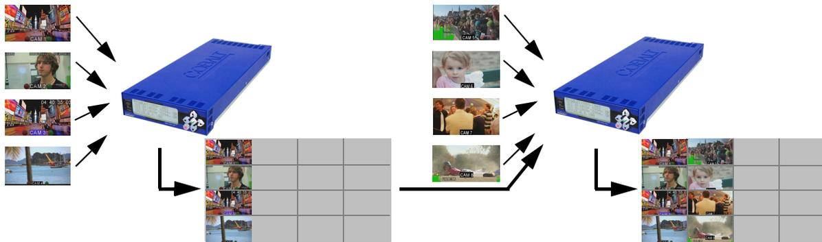
The cascade output (consisting of the four PiP images and a full-size underlay) can be sent to another BBG-1070-QS as a **cascade** input, serving as an underlay which can accept more PiP insertions.
