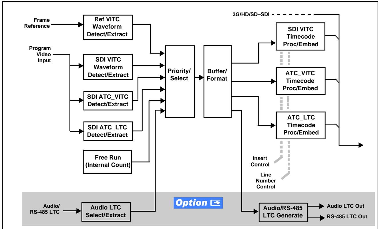
Figure 1-3 Timecode Processor
