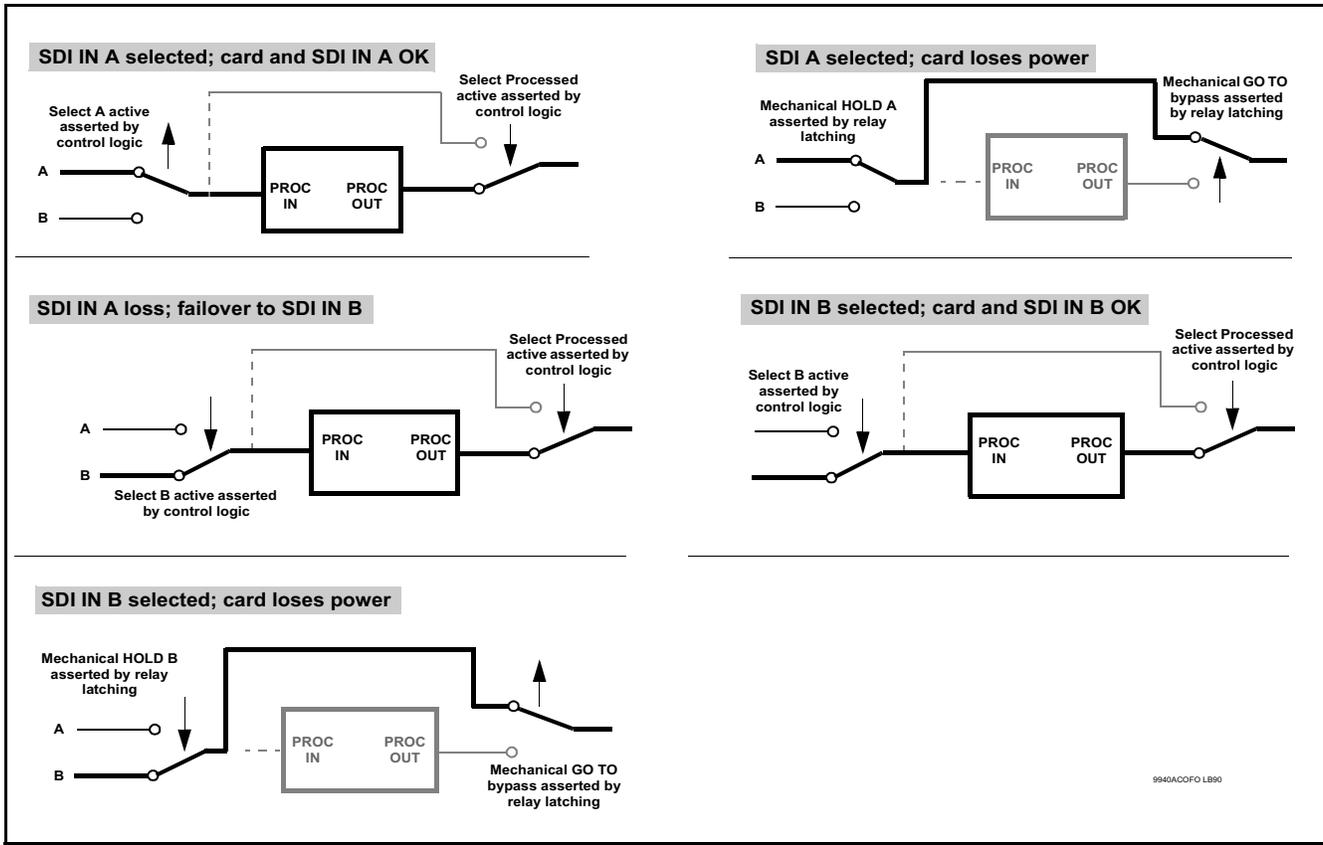
Figure 1-2 Auto-Changeover Function and Example Signal Flow
