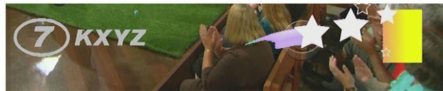
**Key Alpha** setting, when increased, increases the opacity of the key/fill. In the example to the right, progressively increasing the alpha setting increases the key/fill opacity.
