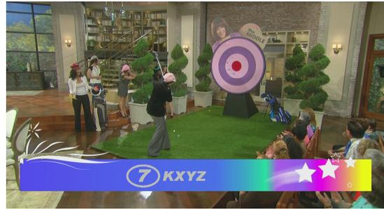
**Key Threshold** setting, when reduced, more readily allows the key/fill input to assert itself over more variations of program video luma levels. In the example to the right, progressively reducing the threshold setting allows more of the key/fill to assert itself over the program video.
