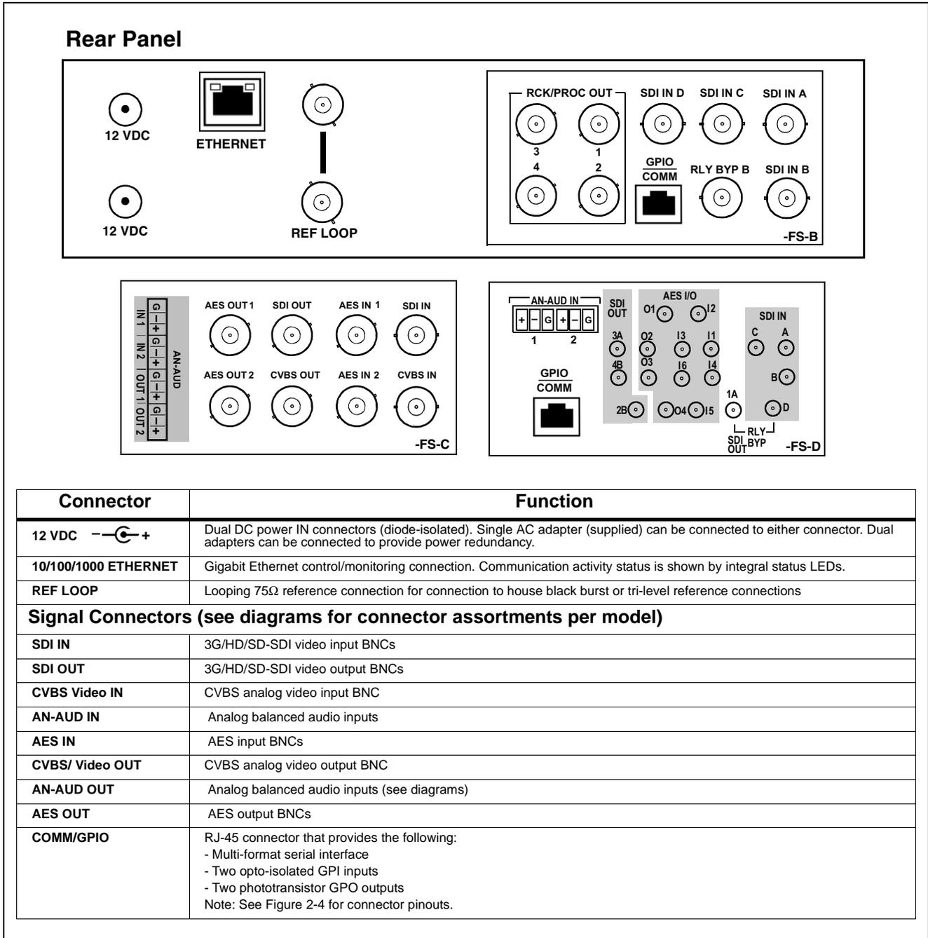
Figure 2-3 BBG-1022-FS Rear Panel Connectors
