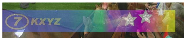
When both settings are optimized, the key/fill appears consistent in opacity and free from edge distortions or graphic bleed lines appearing in the image.
