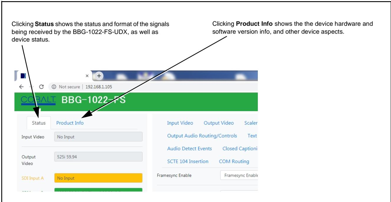
**Figure 3-6 Typical Web GUI Device Info/Status Utility**
