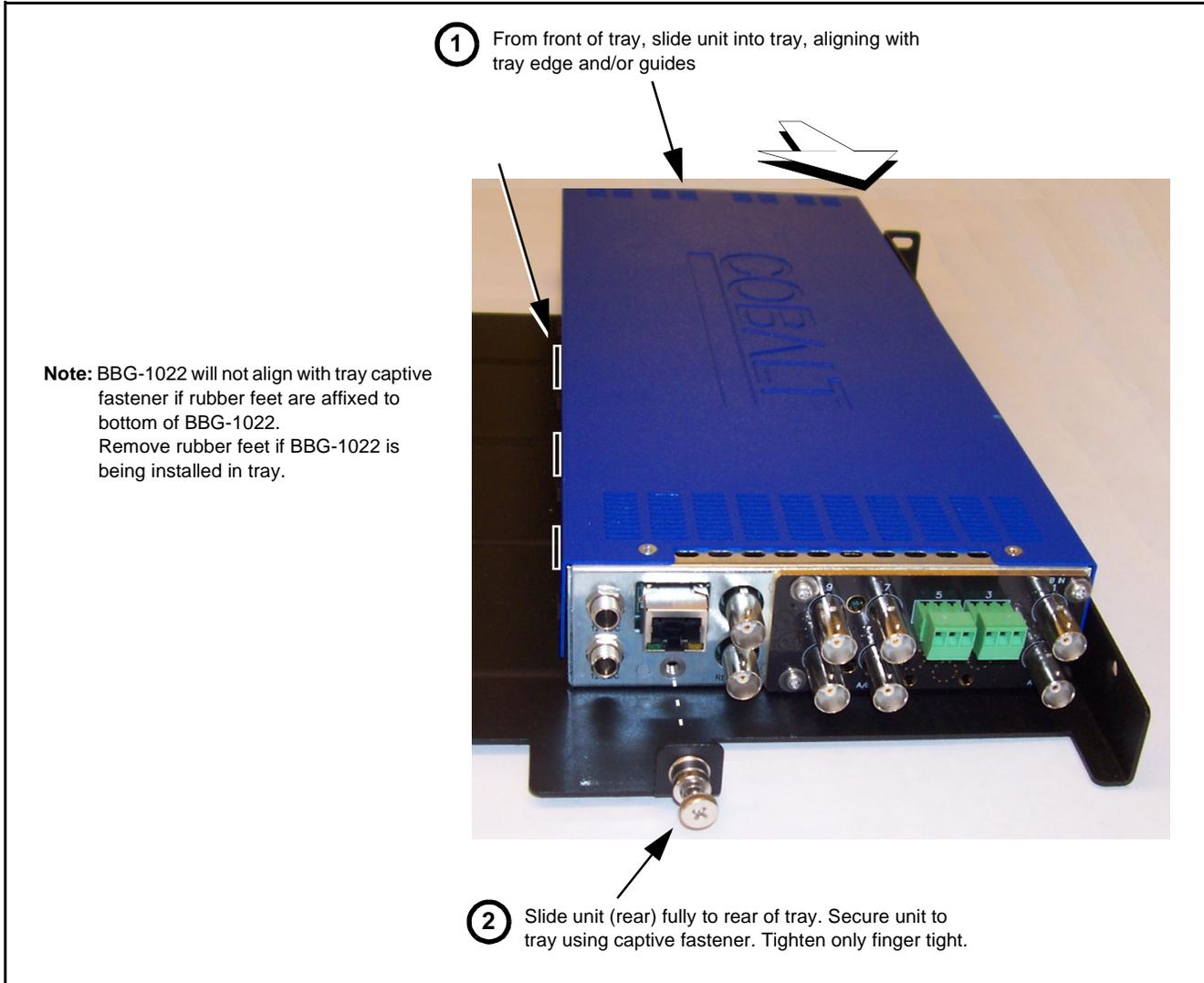
*Figure 2-1 Mounting BBG-1022-FS Using Frame Mounting Tray*
