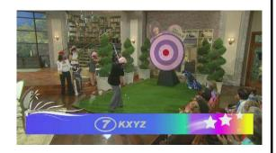
Key Threshold setting, when reduced, more readily allows the key/fill input to assert itself over more variations of program video luma levels. In the example to the right, progressively reducing the threshold setting allows more of the key/fill to assert iteslf over the program video.
