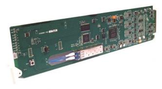
The Cobalt® 9410DA-2EO 3G/HD/SD-SDI / ASI / MADI Fiber Dual EO Transport/Distribution Amplifier with Full-Flexibility Crosspoint provides a card-based solution for high-density conversion from coax to fiber (with two independent EO channels), as well as coaxial distribution. The 9410DA-2EO is multi-rate, and supports SDI and ASI/DVB on all inputs and outputs with non-inverting outputs.
