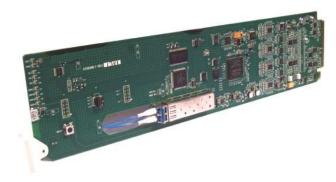
The Cobalt® 9410DA-20E 3G/HD/SD-SDI / ASI / MADI Fiber Dual 0E Transport/Distribution Amplifier with Full-Flexibility Crosspoint provides a card-based solution for high-density conversion from fiber to coax (with two independent 0E channels), as well as coaxial distribution. The 9410DA-20E is multi-rate, and supports SDI and ASI/DVB on all inputs and outputs with non-inverting outputs.
