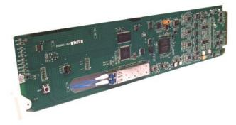
The Cobalt® 9410DA-0E 3G/HD/SD-SDI / ASI / MADI Fiber 0E Transport/Distribution Amplifier with Full-Flexibility Crosspoint provides a card-based solution for high-density conversion from fiber to coax, as well as coaxial distribution. The 9410DA-0E is multi-rate, and supports SDI and ASI/DVB on all inputs and outputs with non-inverting outputs.
