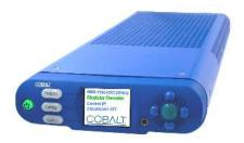
The Cobalt® **BBG-1190-DEC-MPEG Standalone MPEG4 AVC and MPEG2 Decoder** with ASI and IP Inputs and SDI Outputs provides a high performance real-time MPEG-2 and MPEG-4 SD and HD video decoding solution. Its design is practically future proof and decodes traditional video formats such as UDP and RTP (MPEG Transport Stream) as well as Internet and Mobile formats such as RTMP (Adobe® Flash) and HLS (Apple® HTTP Live Streaming).
