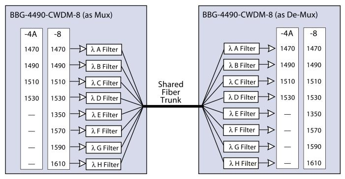
BBG-4490-CWDM offers several choices in fiber wavelength (channel) capacity, ranging from 4-channel to 18-channel (shown here are the 4- and 8-channel models; see Ordering Info that lists wavelength divisions for 12-, 16-, and 18-channel models). All units can be used as a mux or a de-mux unit. Two units (min) are required for a complete mux / de-mux setup.
