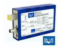
The Blue Box™ **BBG F-T0-H Fiber-To-HDMI** throw-down converter unit is a new part of the Blue Box Group™ of compact, rugged, and portable converter boxes. BBG F-T0-H offers a compact throwdown unit that provides direct fiber-To-HDMI conversion and much more.
