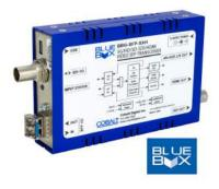
The Blue Box BBG-SFP-SXH 3G/HD/SD-SDI / ASI Reconfigurable Video SFP Transceiver with Externally-Accessible SFP Module throw-down converter unit is a part of the Blue Box Group™ of compact, rugged, and portable converter boxes.
