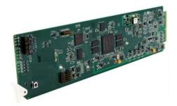
The highly flexible 9363 Multi-Format Reference Generator generates four reference signal pairs that are independently configurable as composite black burst or tri-level reference sources. Each output can be any industry standard rate related to a received input reference source, or can be generated using the card's internal clocking source. Timing for each output pair can be independently offset (in vertical lines or horizontal pixels) from the received reference or internal clock.
