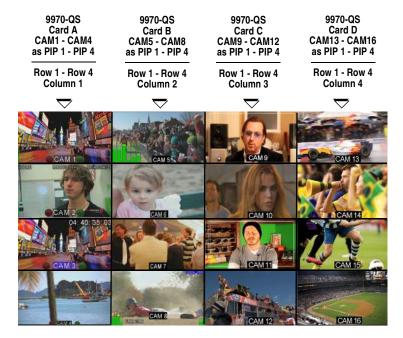
7. Once set in the grid, a PIP is not necessarily locked into its initial position. Any PIP in the cascade can be resized or repositioned into anywhere on the overall output image as desired.
