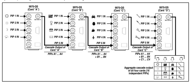
Using the cascade mode on successive downstream cards, the PIP 5 input is configured to serve as a full-size underlay. The downstream-card PIP 1 thru PIP 4 inputs are then inserted as overlays placed on top of the cascade underlay. In this manner, added PIPs are positioned over the imported underlay resulting in a combined image of the imported underlay PIPs and the locally added PIPs.
