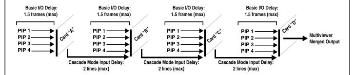
To take advantage of the cascade-mode bypassing/low-latency features, the following should be observed:
