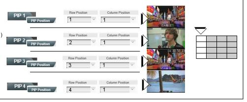
5. On Card B (which is now receiving the cascaded Card A PIP 1 thru PIP 4 positioned in column 1 as an underlay), the Card B PIPs can now be inserted and positioned. In this example, CAM5 thru CAM8 images (using Card B inputs PIP 1 thru PIP 4) are being directed to the cells just across from CAM1 thru CAM4 in column 2 using the Card B Row Position and Column Position drop-downs as shown below.
