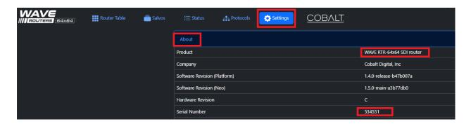
As shown in Figure 1, select **Settings**, scroll down and select **About**. Confirm you see the WAVE Router you intend to update. Select the **Administration** drop-down menu bar. Under **File Upload**, select **File** and find the *downloaded file* on your computer. Once the correct file is found, select it and choose **Upload**. The system will install the new firmware.
