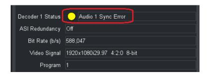
If this alarm is raised, it may be possible to clear this situation by increasing the **Decoder Delay** until the problem clears. Note that changing the **Decoder Delay** causes the channel to restart.
