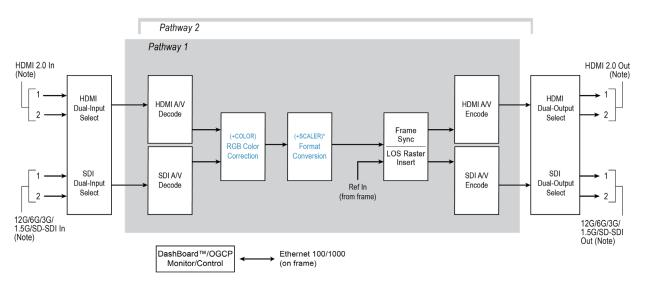
Note: Inputs can be selected from up to 2 discrete HDMI and 2 discrete SDI inputs. Dual simultaneous path processing is available with pathway 2 offering same features/functions as shown for nathway 1.
